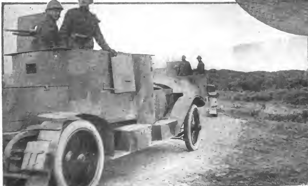
Left—A good rear view of the Belgian armored cars, showing how the rear tires are protected from puncture by bullets. The cars are shown here advancing toward the firing line at a rapid pace
